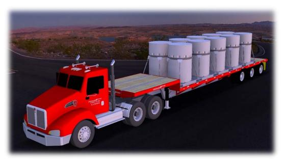
Fig. 3. Typical OPTIMUS<sup>TM</sup>-L Package Transport Configuration
