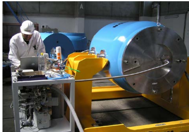
Fig. 3. Cask prepared for loading onto the storage pool
