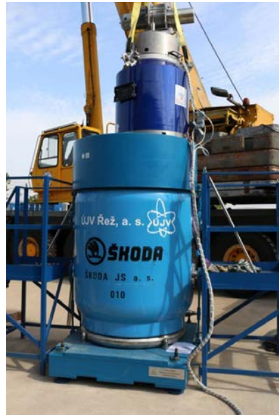
Fig. 23. ŠKODA MNSR cask with transfer cask
