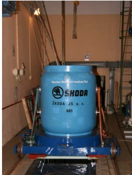
Fig. 3. Cask prepared for loading onto the storage pool
