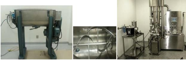
Figure 3: Left - ribbon blender; center - inside ribbon blender; right - granulator
